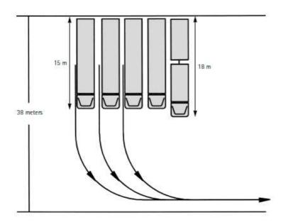
The parking and manoeuvring space in front of the dock should be twice the size of the largest truck adding two extra meters, e.g. 18 meter long trailers needs 38 meters.
