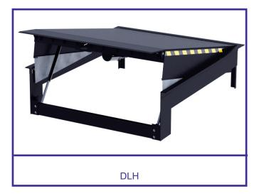
The DLH dock leveller is operated with only one push button. By keeping the push button pressed, the platform will go up from its rest position, when the highest point is reached, the lip will swing out. When the push button is released, the platform and lip will descend automatically to the level of the vehicle bed.
